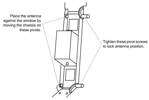
Figure 3-8. Mechanical Window Antenna Pivot Screws
