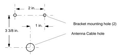
Figure 3-13. Hole Spacing
