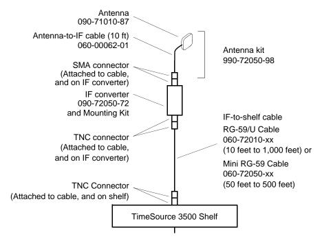
Figure 3-9. Self-Adhesive Window Antenna-to-Shelf Cabling
