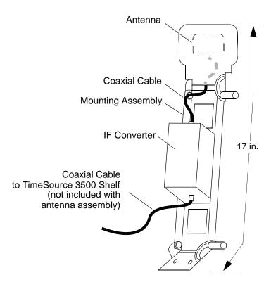
Figure 1-4. Mechanical Window Antenna
