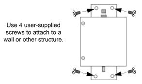
Figure 3-11. Attaching the IF Converter
