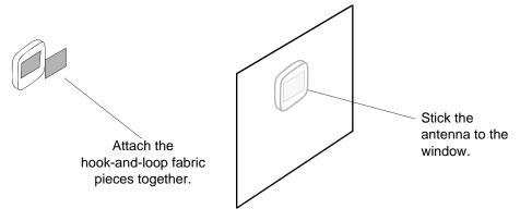
Figure 3-10. Attaching the Self-Adhesive Window Antenna to a Window
