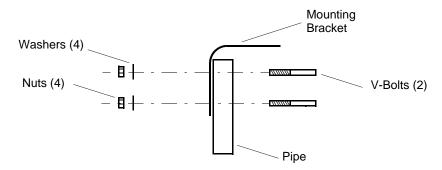
Figure 3-2. Mounting Antenna Bracket to a Pipe
