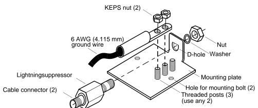
27. If the lightning suppressor was not mounted directly to a valid earth ground, crimp a length of 6 AWG (4.115 mm) ground cable to the two-hole terminal, slide the terminal over two of the three threaded posts on the lightning suppressor mounting plate, and attach the terminal to the mounting plate with two KEPS nuts. Use the two posts that allow the least bending of the 6 AWG (4.115 mm) ground cable.
