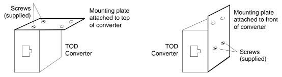
Figure 3-23. RS-422-to-RS-232 TOD Converter Mounting Plate
