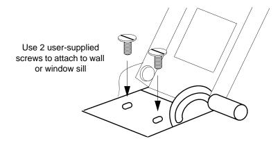
Figure 3-7. Attaching the Mechanical Window Antenna
