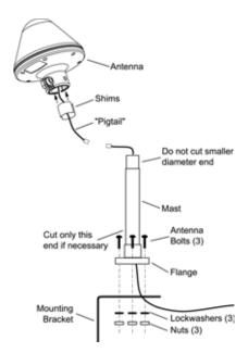
Figure 3-4. Antenna Mast Assembly
