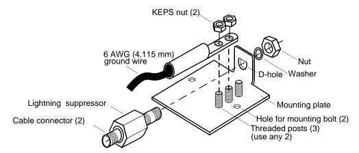
Figure 3-5. Mounting the Lightning Suppressor
