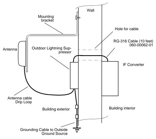
Figure 3-15. Wall Antenna Outdoor Lightning Suppressor Mounting
