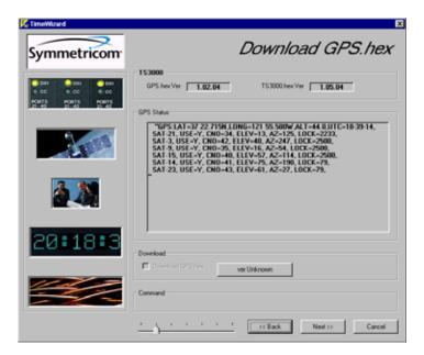
The versions of the GPS.hex and TS3000.hex firmware that are currently installed in the TimeSource are shown in the GPS.hex Ver and TS3000.hex Ver fields. Current satellite information is shown in the GPS Status field.
