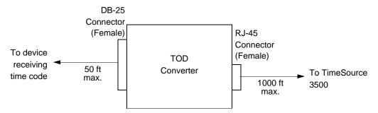
Figure 3-24. RS-422-to-RS-232 TOD Converter Connections
