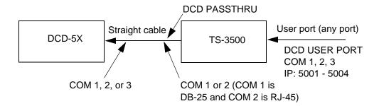
Figure 1-9. TimeSource 3500 Passthrough Function
