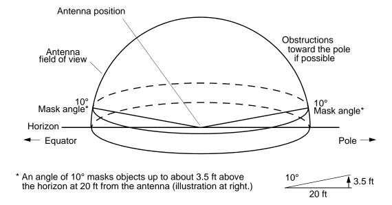
Figure 2-1. Antenna Field of View
