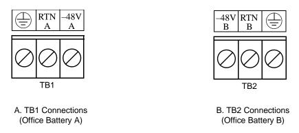
Figure 3-19. Battery Connections
