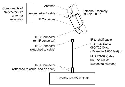
Figure 3-6. Mechanical Window Antenna-to-Shelf Cabling
