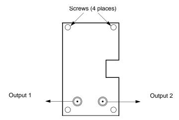
Figure 3-22. IRIG-B TOD BNC Output Connections
