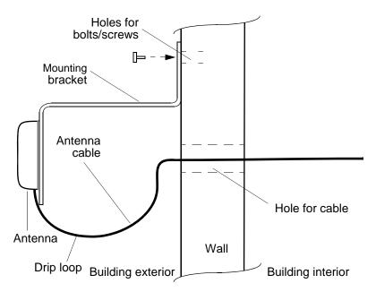
Figure 3-14. Wall Antenna Mounting
