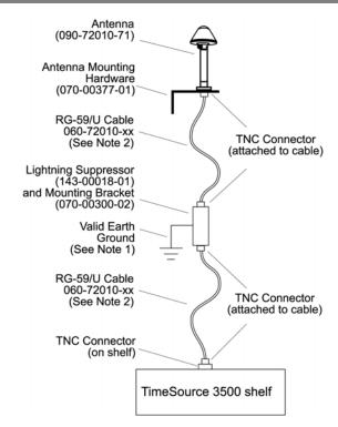
Figure 3-1. Roof Antenna-to-Shelf Cabling
