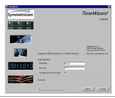
6. The version of TimeWizard that is installed is indicated at the top right of the screen. The progress indicator at the bottom of the screen shows which of the seven screens you are currently viewing.
