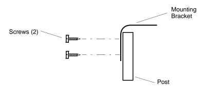
Figure 3-3. Mounting Antenna Bracket to a Wood Post
